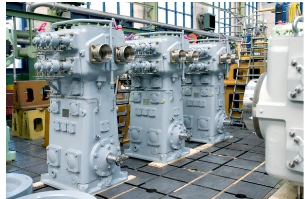
Figure 5: LPG BOG Laby® Compressor 2K160-2A
